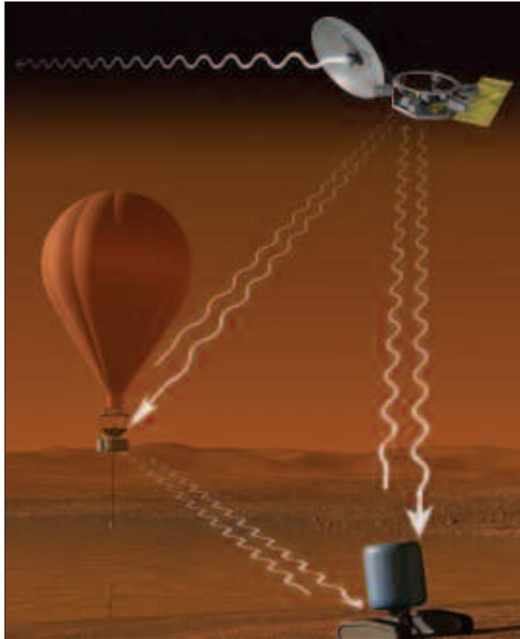
ploy surface packages, representing a third tier of exploration platform. These might include the network of sensors, or sensor web, needed to probe subsurface structure with seismic or electromagnetic waves. Data from these sensors might be relayed to Earth via the atmospheric platform, orbiter, or both.
